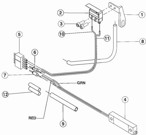
MODEL 8 IPB 080803 LIMIT SWITCH-TRIM POT ASSEMBLY (M8-2000, M8-4000 AND M8-6625)
