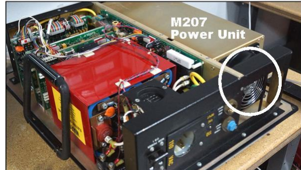
Fig. 3: Dual exhaust fans (circled in top photo) draw air into and out of the M217, providing air flow throughout the interior. The M207 (pictured above) has a single fan providing direct air flow for the power unit only.
