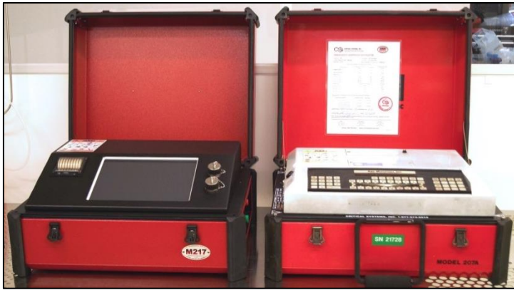
Fig. 1: The footprint of the M217 is the same as the M207, although it is 13 lbs. lighter (66 lbs. vs. 79 lbs.).
