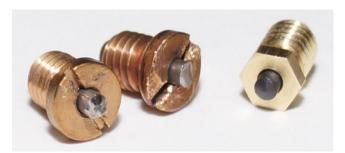
The flat-blade slot in standard home pin bushings provide less support for the home pin. This allows the home pin to flex and wear unevenly. Hex head design gives consistent home pin support, minimizing pin damage.
