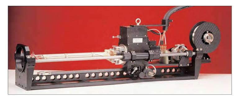
The Model 94 is a rugged weld head designed for high production spiral or step ID cladding and groove welding on small diameter pipes, fittings and vessel inlet/outlets, using the GTAW (TIG) process with cold wire feed. The Model 94 is a stable, precise and repeatable platform for manipulating many different torches for welding and cladding operations.
